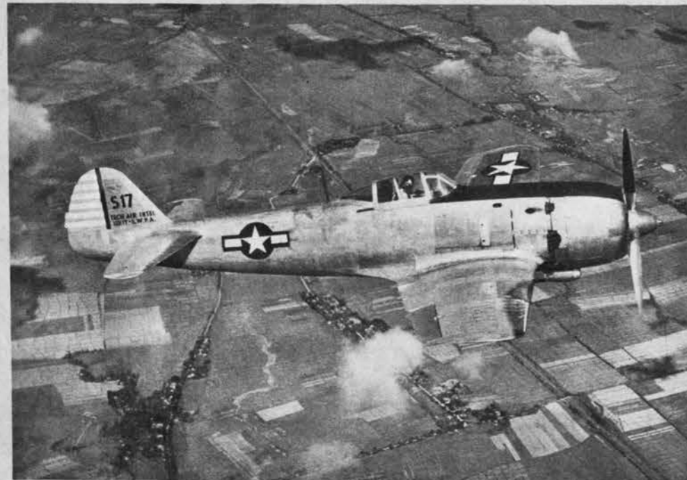
Frank's wing with straight leading edge, blunted tips often causes it to be reported as Oscar. In beam view (below) long slender fuselage shows family relationship to older fighter.
